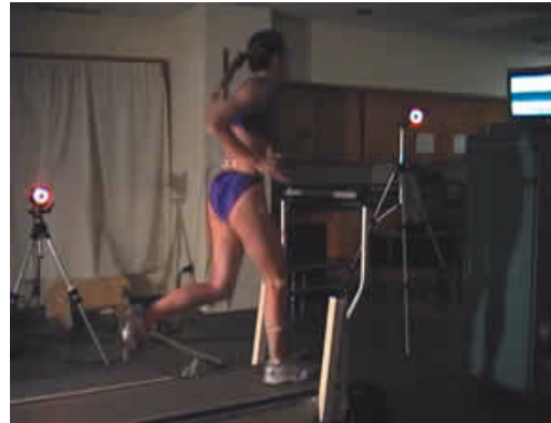
Figure 1: MC running on the treadmill with retro-reflective markers placed on her pelvis, thighs, shanks, and feet. A video monitor (right) was provided for real-time feedback.
