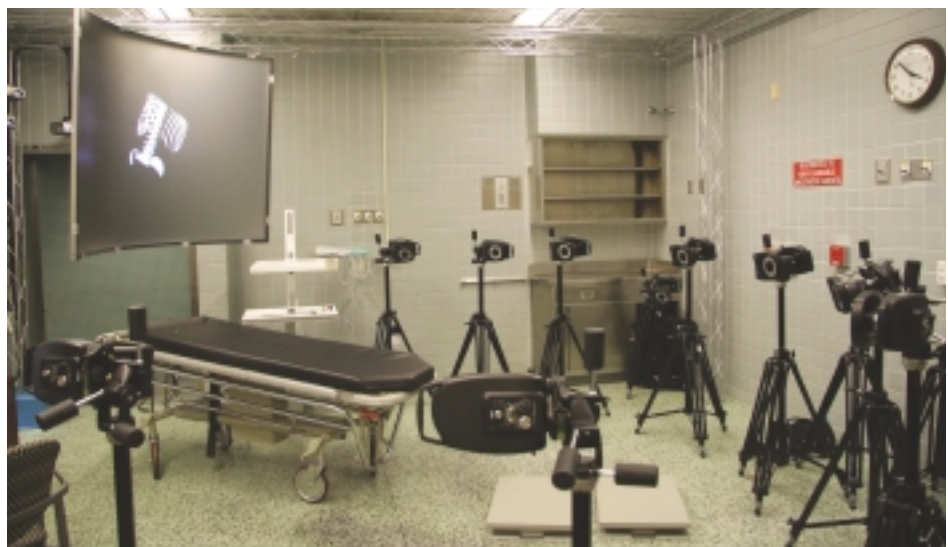
Twelve Vicon MX cameras are used to track the surgeon in front of a high-resolution distributed display system.
