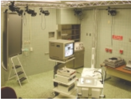
Partial view of the ergonomics laboratory, showing Vicon MX cameras mounted on truss system, trainer station, and display systems.
