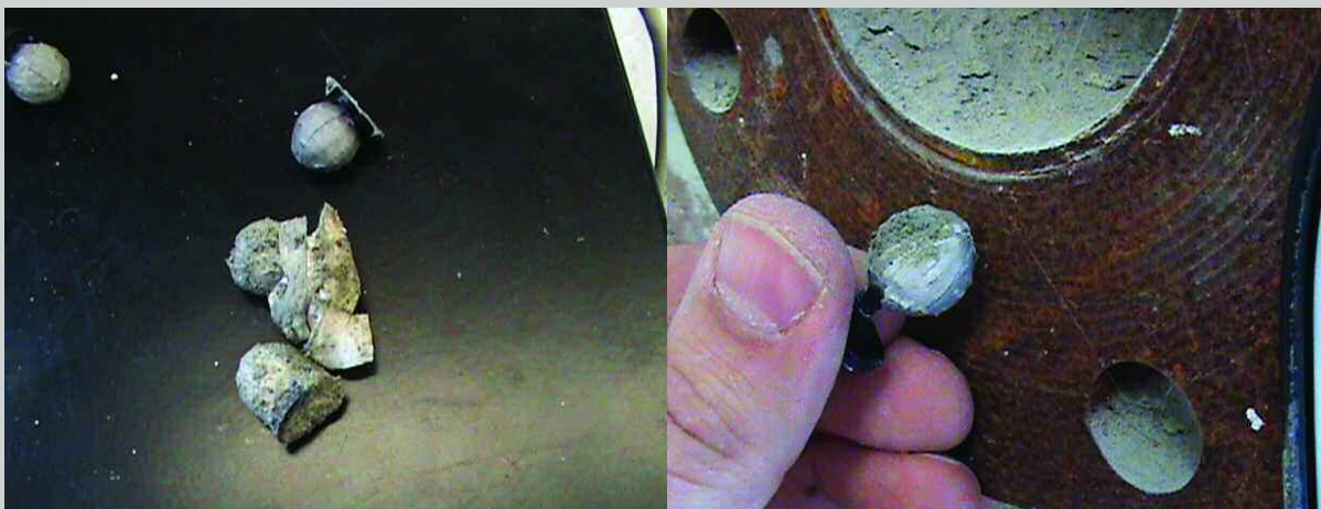
← Markers that accumulated mortar during the data collection
